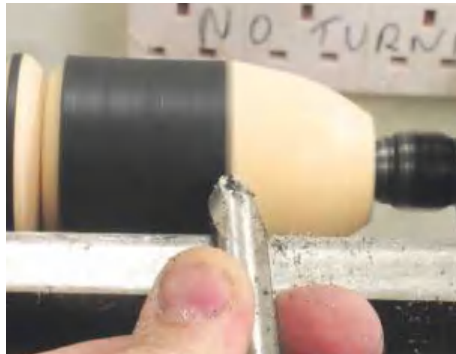
▲ Pic.10 To round over the end of the spindle, start with the bevel on the wood in a position where the tool will start cutting with the minimum movement required
